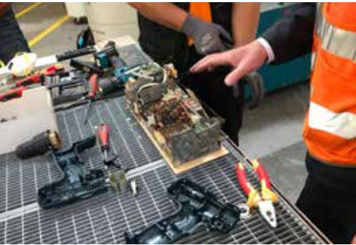
Manual pre-dismantling offers advantages for raw material recovery.
