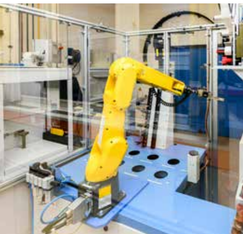
This robot analyzes stamping samples fully automatically.
